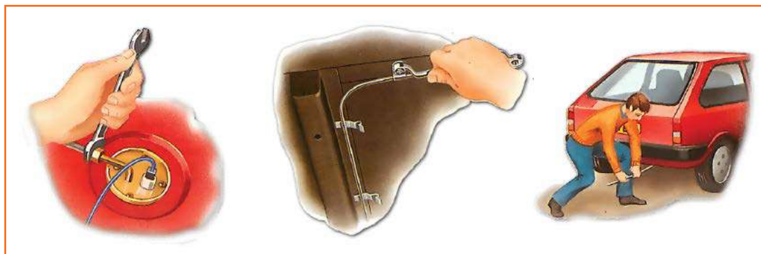
Fig 4.3.23: Replacing fuel pipe
