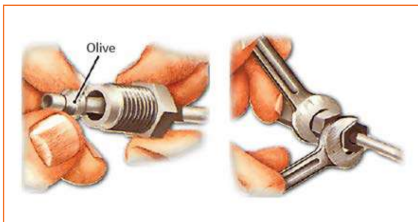
Fig 4.3.24: Replacing an olive
