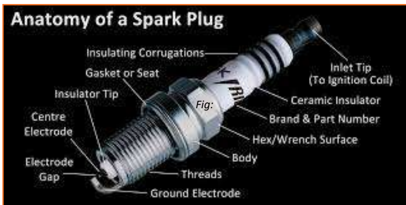
Fig 4.3.288: Spark plug parts
