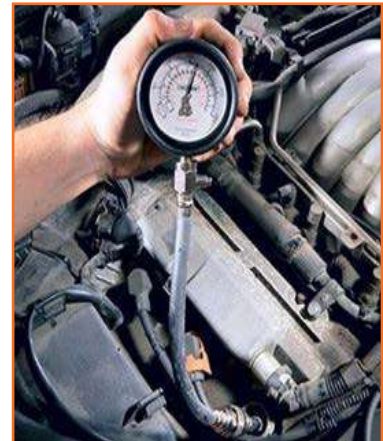
Fig 4.3.13: Engine compression testing
