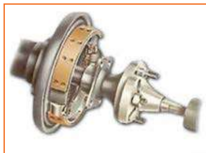
Fig 4.3.106: Removing half shaft
