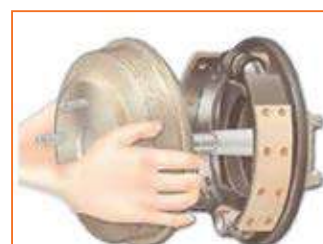
Fig 4.3.205: Pull the drum off by hand
