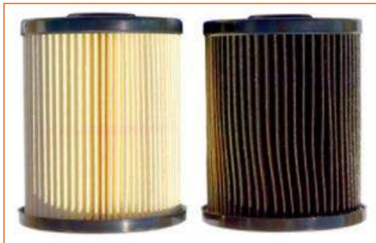
Fig 4.3.28: Clean and dirty diesel filters
