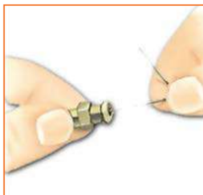
Fig 5.2.60: Carefully poke the nipple clear with a thin wire
