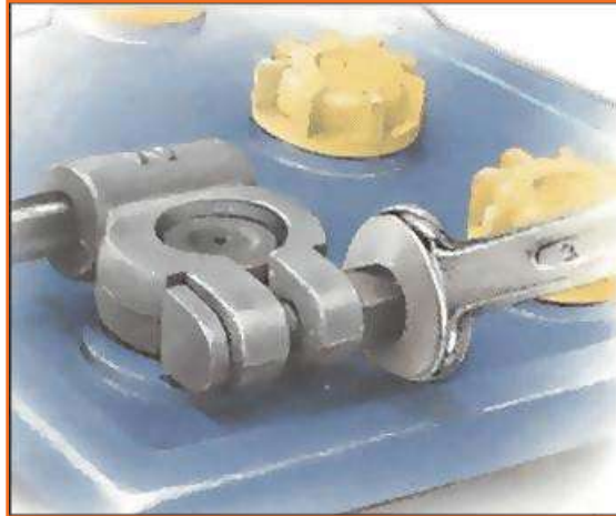
Fig 4.3.217: Inspection of battery
