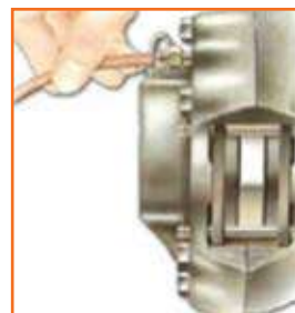
Fig 5.2.57: check the bleeding process 2
