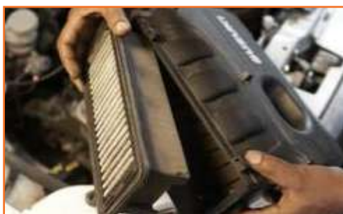
Fig 5.2.2: Removal of filter element
