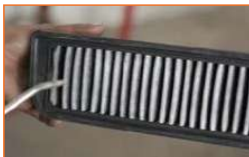
Fig 5.2.3: Cleaning with compressed air
