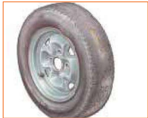
Fig 4.3.112: Sign of tyre wear and damage
