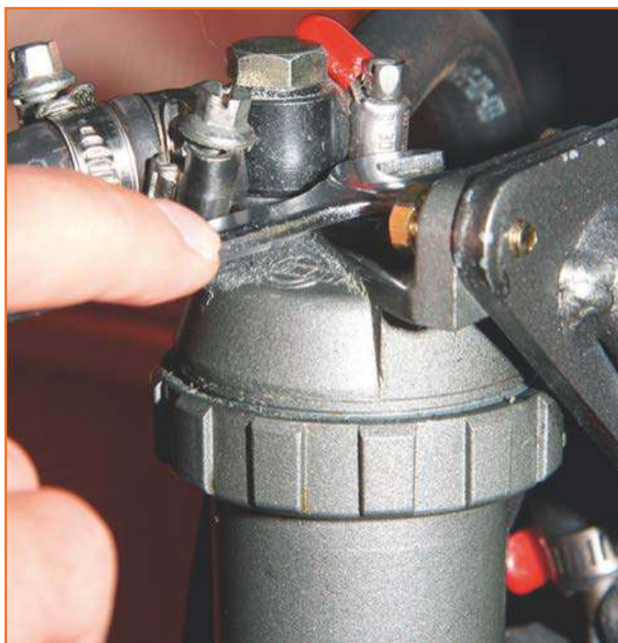
Fig 5.2.12: Air bleeding from fuel system
