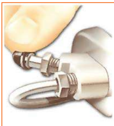
Fig 5.2.46: Releasing the bleed nipple
