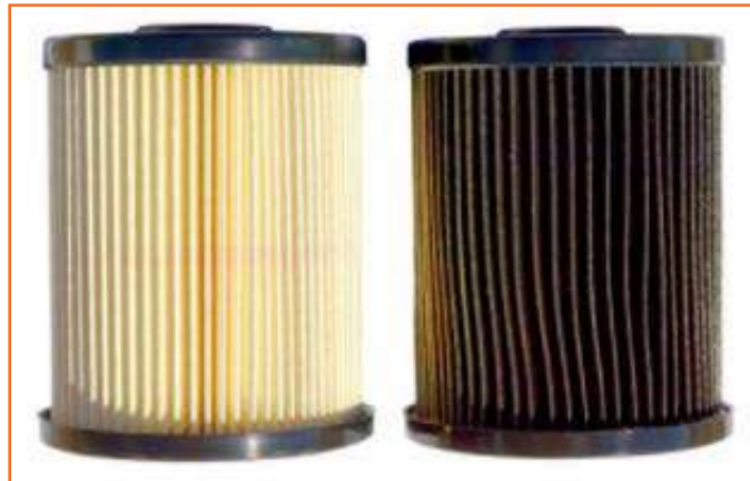
Fig 5.2.11: Clean and dirty diesel filters
