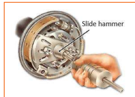
Fig 4.3.101: Removing half shaft
