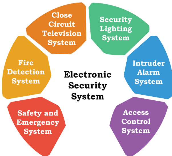
Fig. 3.5: Components of an electronic security system
